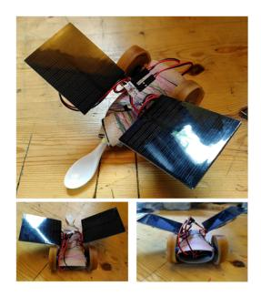
"The Solar Drawing Machine" is a second prototype under development. Learners are given a base model that is powered entirely by the sun which they can modify to explore different possibilities. The speed of the machine's rotation varies according to the solar
